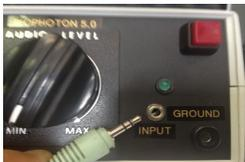
Connect the **3.5mm jack to INPUT port** for adding custom programs and/or frequencies included with the 5.0 upgrade. 4.0 version can be upgraded to 5.0. ONLY use low level voltage inputs, such as a CD player, audio tuner, Light Box, etc..
