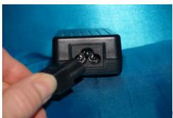
Connect the power cord into transformer for power supply source.
