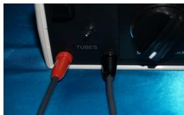
The **sending** glass tube electrode is connected into the **red jack**. The **"receiving"** glass tube electrode is connected into the **black jack**.
