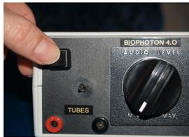
**Push the black push on/off button**, on the upper left, front corner next. This powers the electrodes. The **Amber** (neon) lamp below this switch will glow in an on/off manner and the tubes will light with a color.
