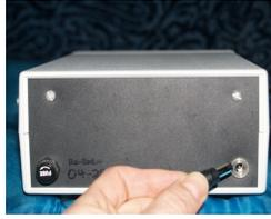
**Connect power supply** into DC jack located behind unit, on right side.
