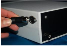
Connect Sound Probe into receptacle along right side, back of unit.
