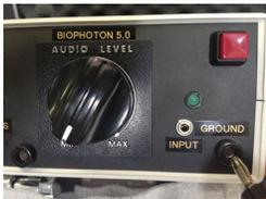
Connect the **copper sided Ground Plate black/male plug** into the black female banana jack on front; lower right corner, (under red button) marked "Ground". (For Ground Plate **ONLY!** **No Tubes should ever be plugged into this jack**)
