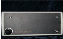
**The 1 1/2Amp 250v fuse** is located on the lower left, backside of the unit, in a quick release fuse holder. This unit draws very little energy from the power source and the fuse may never have to be replaced. High voltage output without tubes plugged in, faulty transformer or defect in circuit board may cause fuse to blow.
